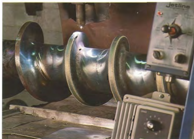
PTA and traditional welding are done on the premises. Colmonoy #56 hard facing is being applied to a 12" densifying screw.
